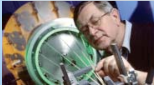
RESEARCH MAKES IT POSSIBLE - HIGH TEMPERATURE SUPRA-CONDUCTORS ARE ATTACHED TO A CABLE THAT CAN BE USED FOR APPLICATIONS USING MAINS CURRENT.
